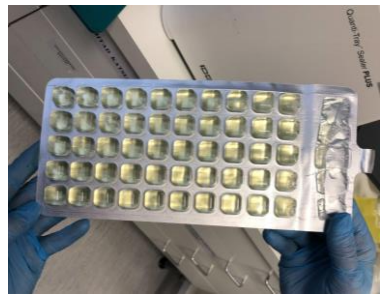
Quanti-Tray Sealer Plus masinaga suletud Quanti-Tray kott, milles on basseinivee proov. (Foto autor: Elis Kägo)
